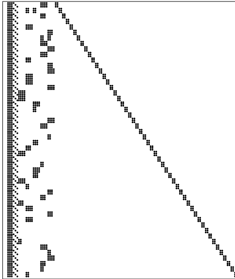
Figure 4: Representative sparsity pattern of the HT Jacobian, adapted from the ADBench benchmark paper [9]. Black entries are structurally nonzero, while white entries are zero.
