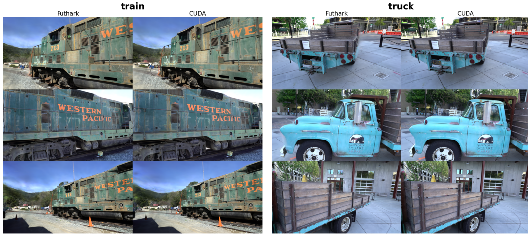
Figure 3.2: Qualitative Comparison: A comparison between the Futhark and CUDA renderer outputs after 30k training iterations. The left-hand column of images is from the train dataset, whereas the right-hand images are from the truck dataset. Futhark renders look a little fuzzy around the edges of some objects because of the use of the for loop in the pixel color calculation. All images are from the testing set, meaning that the scene was not trained on them.
