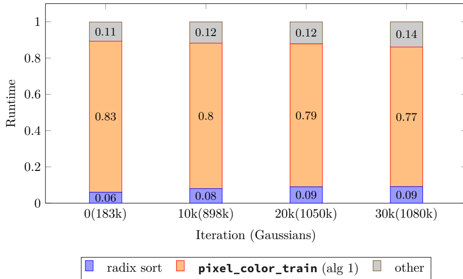
Figure 3.3: Profiling results: The fraction of runtime spent on each function of my Futhark rasterizer while training the “Train” scene from Tanks and Temples[16]. In this graphic, pixel_color_train corresponds with the pixel_color_train function described in section 3.2.2. These numbers were generated by resuming training from a checkpoint with the command line argument --futhark_profile 200 given to the train.py file. The performance of the Futhark rasterizer was then profiled for the next 200 training iterations, and the results were processed with futhark profile .
